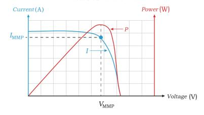
Maximum Power Point Tracking is electronic tracking. The charge controller looks at the output of the panels and compares it to the battery voltage. It then figures out what is the best power that the panel can put out to charge the battery. It takes this and converts it to best voltage to get maximum AMPS into the battery.
