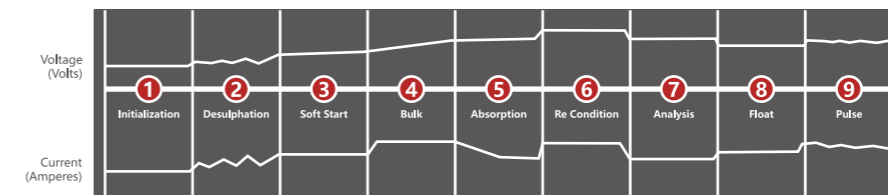
Automatic and High Frequency 9-Stage Charging Curve ■ For all smart charger apply on Gel and normal battery
