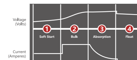
Automatic and High Frequency 4-Stage Charging Curve ■ For all smart charger, apply on Gel and normal battery
