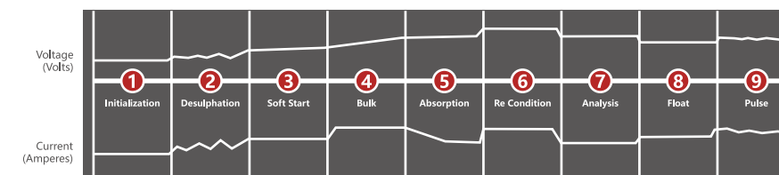
Automatic and High Frequency 9-Stage Charging Curve
